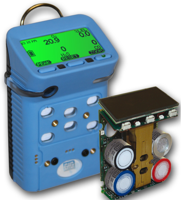
Figure 3: IR CO 2 sensors detect gas as a function of absorbance of infrared light at a specific wavelength
