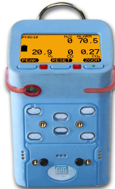
Figure 1: Compact multi-sensor instruments are capable of providing direct CO 2 measurement during confined space and other atmospheric monitoring procedures
