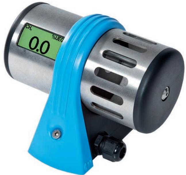
*The IR-29 is a fixed system gas transmitter equipped with an infrared sensor used to measure LEL gas. The IR-29 is certified as an intrinsically safe “Ex i” device for use in Zone 0, gas group IIC, temperature class T4 hazardous locations. The intrinsically safe design does not depend on an explosion proof housing, which reduces noise and improves performance of the IR sensor.*
