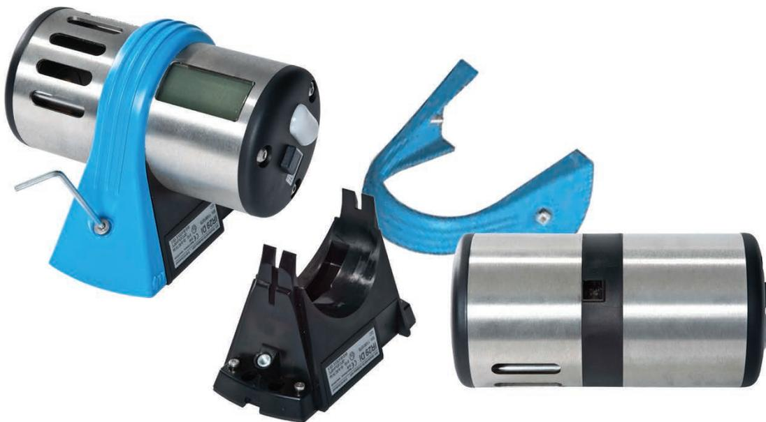
***The sensor head assembly of the low power “Ex i” certified IR-29 transmitter can be removed and replaced even when the transmitter is located in Zone 0, gas group IIC, temperature class T4 hazardous locations. Being able to remove and replace the head without needing to declassify the hazardous location makes it easier to perform maintenance procedures such as calibration and repair.***
