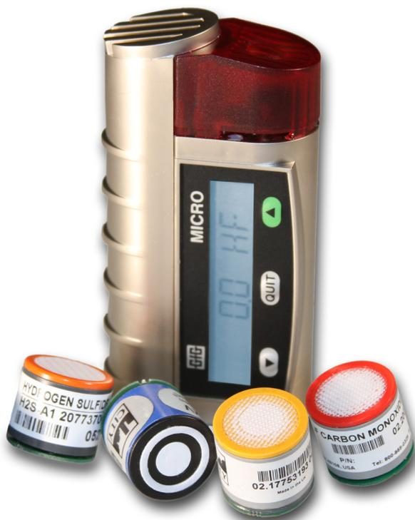
**Sensors used to measure hydrogen fluoride (HF) are dependable and accurate, but require special care during calibration and functional test procedures.**
