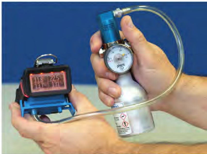
Performing a bump test verifies the alarms are activated and that the instrument properly responds to gas. (photo courtesy GfG Instrumentation, Inc.)
